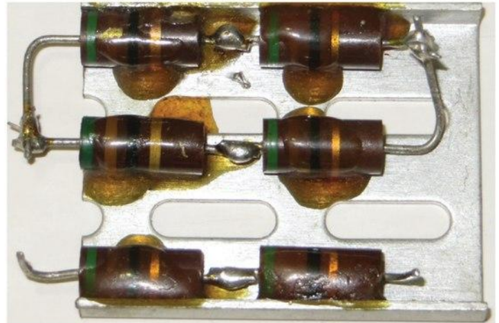
FIGURE 5. An array of one watt resistors on a heat spreader capable of dissipating 10 watts.
